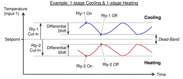
The Dead-Band can not be programmed directly, it is a combination of the Relay Cut-in's and Differential Shift settings.
